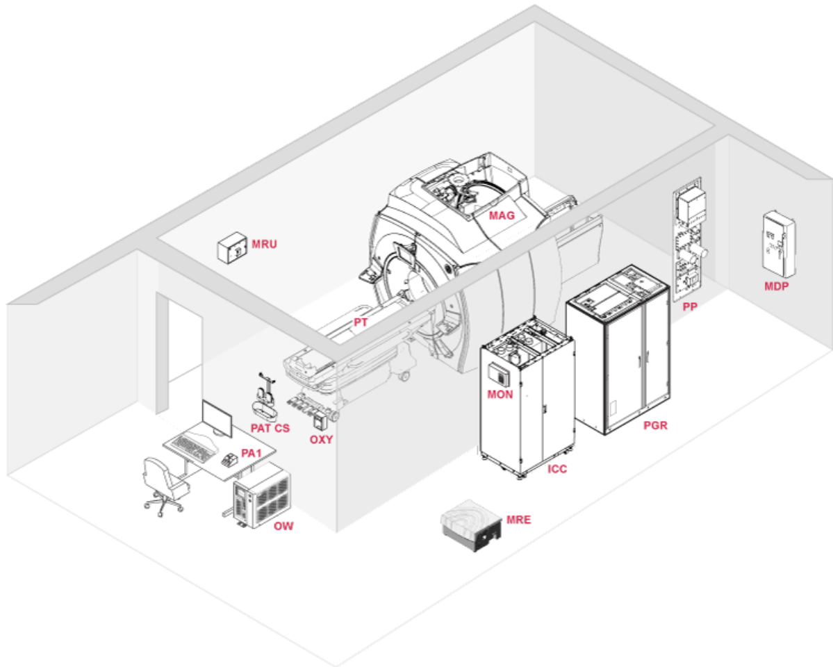
Figure 2-1 System overview (example)
